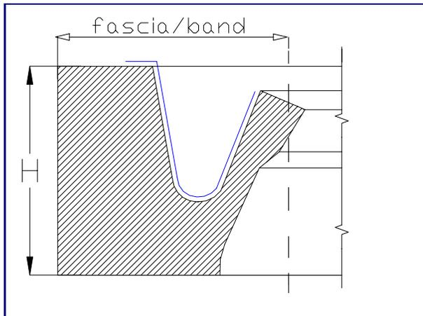
The band is referred to the nominal sizes and is equal to the half of the difference between the OD size and ID size.
