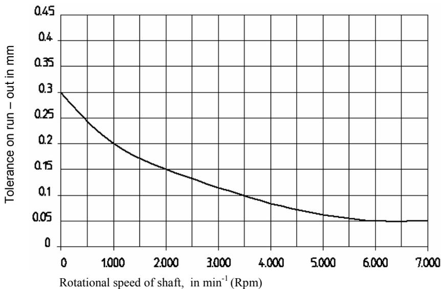
Beyond such limits in coaxiality and alignment we recommend development of a special seal.
